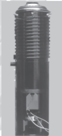
Pressure vessel and axial loading column
